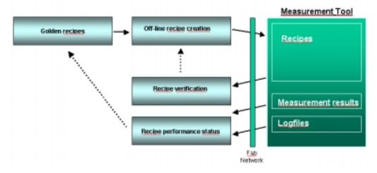
**Figure 5.** The Global Approach to recipe management integrates Golden Recipes, Offline Recipe creation, and JIT recipe creation, with a Recipe feedback mechanism for a maintaining optimum overlay recipe performance.
